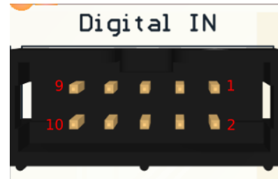
6 Fig. Digital In connector pin numbering
