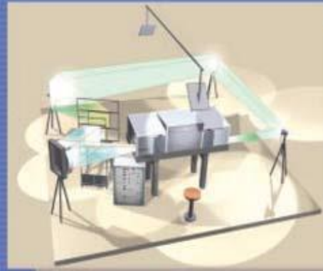
4. Shooting the copy - H1 beam comes from the left, H2 from the right
