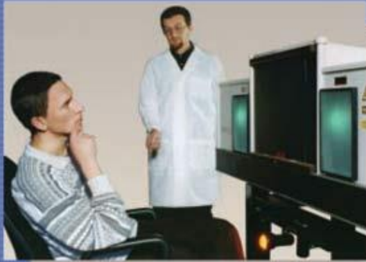
A 3D portrait is made with an HS Mini-Studio (2 diffusers provide subject illumination)
