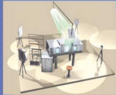
2. Exposure: 2 illuminating and 1 overhead reference beams
