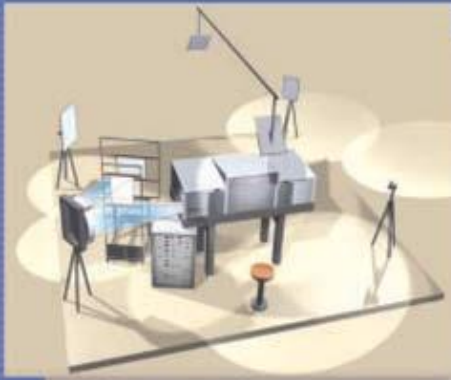
3. Adjusting the copy hologram for final image position and framing
