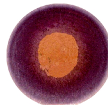
Typical near field distribution High Energy mode - G5J, E = 2J - 1053 nm
